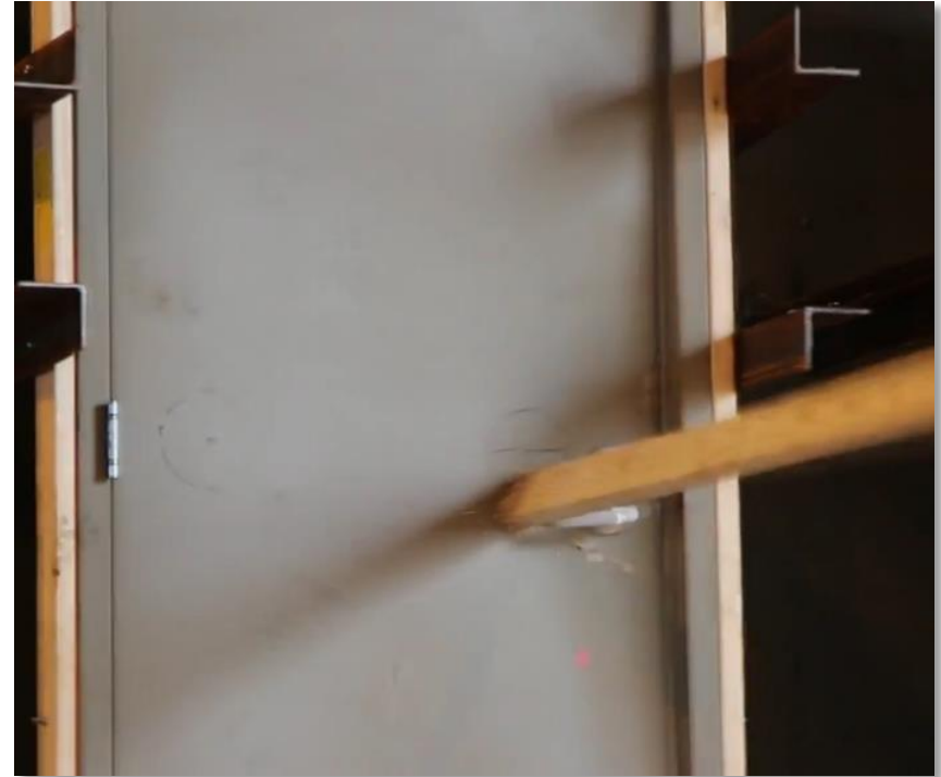
Test footage of steel door withstanding three projectiles at 100mph
