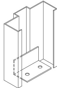
**MASONRY STRAP & STIRRUP:** A fixed metal device used to secure the frame to new masonry walls.
