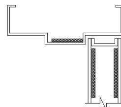
**PARALLEL ARM:** Reinforcing in soffit of frame header or transom mullion.
