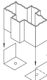
**POURED IN PLACE:** A metal device used to secure a frame to new concrete pour in place wall.
