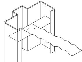
**MASONRY WIRE:** A loose metal device used to secure the frame to new masonry walls.
