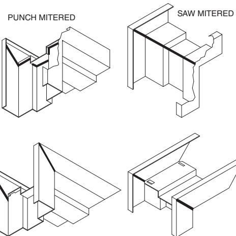
**WELDED, FACE, FRAME:** Comer/perimeter joints shall have a continuous weld at the faces only.
