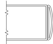
**BULLET RESISTANT:** A hollow metal assembly designed and manufactured to resist penetration by fire arms projectiles.
