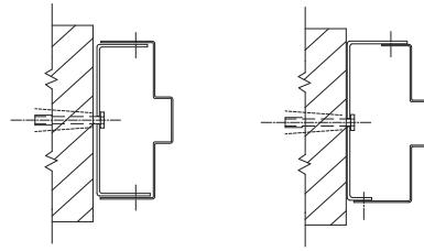
**ROUGH OPENING:** The size of the wall opening into which a frame is to be installed.
