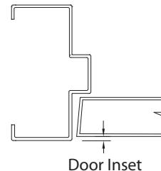
**DOOR OPENING:** The area in a frame product into which a door or doors are installed.
