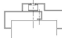
**ANCHOR:** A metal device provided inside of a jamb, head, sill or mullion used to secure the frame to the adjacent structure, such as wall, ceiling or floor. Also referred to as jamb anchor, wall anchor, floor anchor, etc. See listing;
