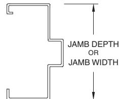
**JAMB EXTENSION:** That portion of a jamb which extends below the level of the floor. See Also **BELOW FLOOR.** (*For additional information, see HMMA TechNote HMMA-810 TN01-03, "Defining Undercuts."*)
