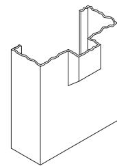
**CUTOUT:** A hole in the hollow metal door or frame to accommodate hardware, light kits, louvers or other options.
