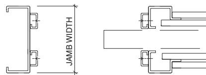
**POCKET DOOR FRAME:** Frame designed to allow a door to slide inside a pocket located within the cavity of a wall.
