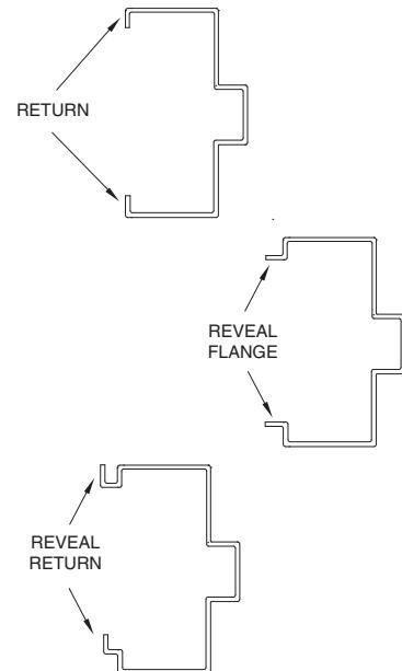
**REVEAL FLANGE:** The element of the frame profile, which extends from the return. Typically formed parallel to the wall.
