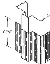
**SPLADE PROFILE:** A frame member where the transition from stop to opposite face is sloped. Also referred to as Hospital or sloped Profile.
