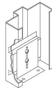
**COMPRESSION:** An adjustable metal device, used to secure, adjust and square a slip on frame.
