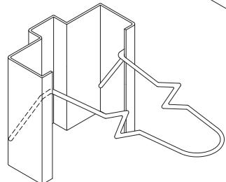
**MULLION:** A metal clip or angle in either 1 or 2 pieces, secured to the floor in which mullion is then positioned over.
