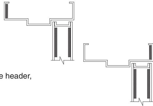
**REGULAR ARM:** Reinforcing in pull side face of frame header, transom mullion, or panel.
