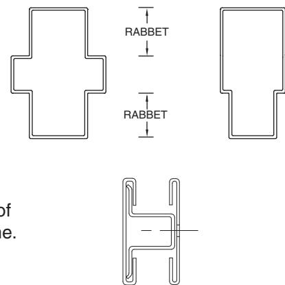
**MUNTIN:** A bar or formed material supporting and separating panes of glass within a door, sidelight, transom, borrowed light, or window frame.
