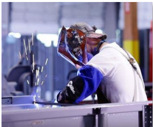
Tack weld a shipping bar
