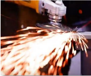
Grind weld level
