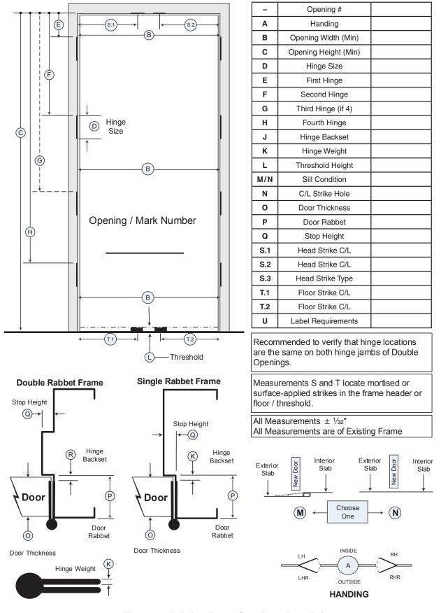
Figure 3 – Existing Frame Opening – Door Pair
