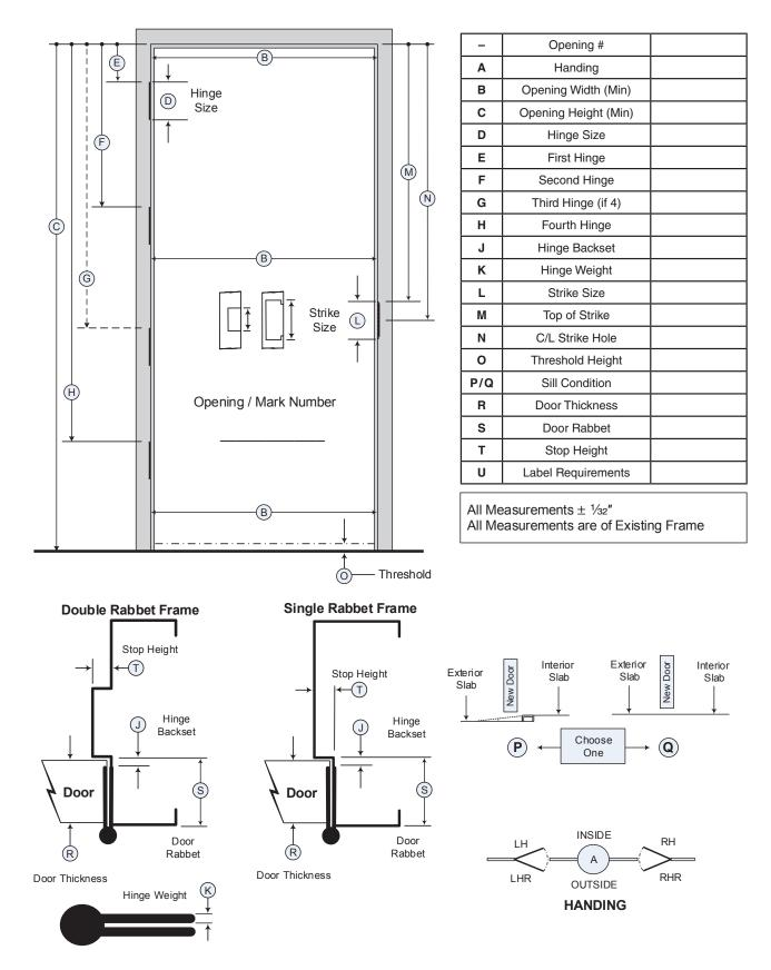
Figure 1 - Existing Frame Opening - Single Door
