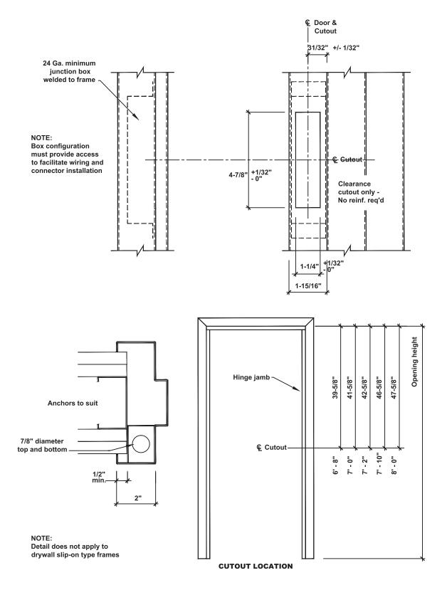
Figure 4 – Electrified Continuous Hinge Preparation on Standard Steel Frame
