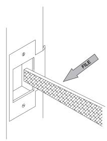
The previously mentioned items should be checked and any problems corrected. If the latch continues to tightly engage the strike, additional clearance can be created by filing the strike or bending the latch bolt lip as shown. However, this should only be done as a final option.
