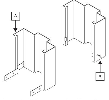
below. Both the "A" and "B" dimensions will be the same when the frames are properly set. However, the frame jambs must be plumb, level, and square with the head of the frame.
