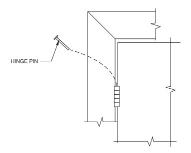
**NOTE:** As always, caution should be exercised when the hinge leaves are not removed. **Excessive** pressure could damage doors/frames. As an alternate reswaging method, the hinge can be removed and clamped in a vise for reswaging.
