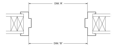
If both jambs are toed in/out, they both should be "squared-up." This can be checked by taking measurements as shown above. Both the "A" and "B" dimensions will be the same when the frames are properly set.
