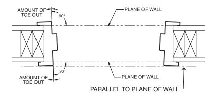
Note that the rabbet surfaces are not 90° to the plane of the wall. This can be checked by placing a straight edge across the face of both jambs.
